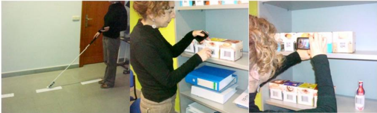
Figure 2: Navigation through RFID and a white cane (left), product recognition by UPC code technology (middle), product recognition by QR-code technology (right) (López-de-Ipina et al., 2011)
